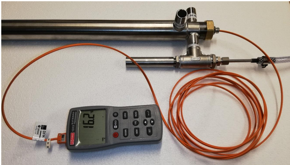
Figure 4 The injector is shown mounted on water-cooled suction pyrometer. Adjust nozzle position of injector to obtain max gas flow (test with a finger at tip of ceramics).
