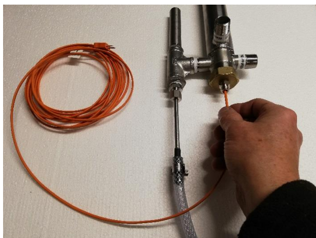
Figure 2 Platinum type R thermocouple protected in a 3 mm diameter ceramic tube is inserted from the rear end through \varnothing 4 mm hole (care: ceramics is fragile, i.e. do not bend or hit anything). Push thermocouple forward until tip is approx. 14-16 cm in front of the water-cooled probe. A small leak of air through the tube where the thermocouple is inserted to prevent dirt to stick on cable a sensor in the water-cooled part of the probe.
