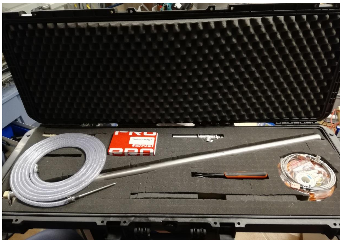
Figure 1 Case with water-cooled suction pyrometer, injector stainless steel (316), calibrated thermometer, type R thermocouple (max. 1500°C), type N thermocouple (max. 1250°C, but works up to 1300°C with reduced life time), ceramic shields and tools.
