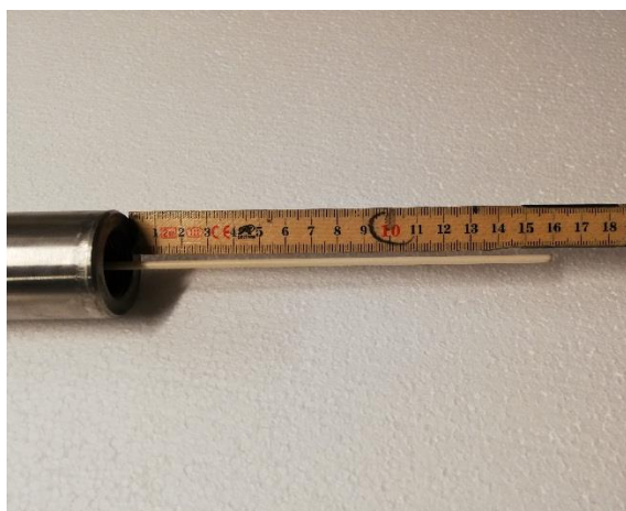
Figure 2 Platinum type R thermocouple protected in a 3 mm diameter ceramic tube is inserted from the rear end through \varnothing 4 mm hole (care: ceramics is fragile, i.e. do not bend or hit anything). Push thermocouple forward until tip is approx. 14-16 cm in front of the water-cooled probe. A small leak of air through the tube where the thermocouple is inserted to prevent dirt to stick on cable a sensor in the water-cooled part of the probe.
