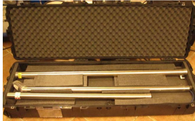
Peli 1770 flight case with water-cooled video probe in 3 parts. Other parts are found below foam. Video probe is approx. 3 m long assembled.
