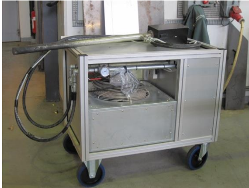
Movable system for burner inspection with fan cooling system. Only power and pressurized air is needed.
