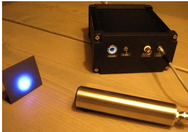
Figure 5 LED power supply and LED Flash Light Pulser. The BNC connector on power supply for measurement of pulse current and width is an option.
